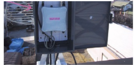
FIGURE 16: Equipment at the main drill site: (a) wireless LAN unit and its antenna; (b) video monitors for a decoder for the portable live video transmitter, a compact helicopter live video transmission system, and an encoder for Shinshu University Hospital and Matsumoto Regional Fire Bureau.
